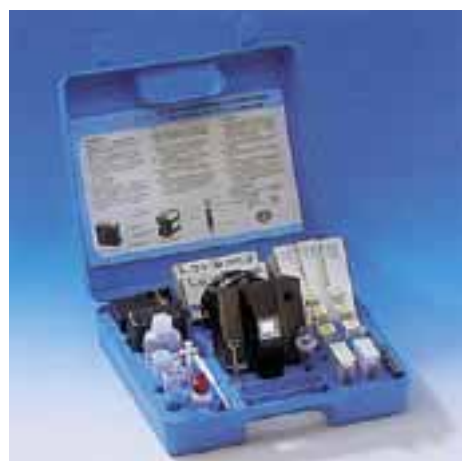
Example of a comparator test kit, together with portable daylight unit and charger (optional extras)
