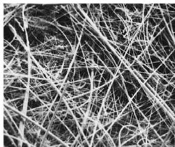
Glass microfiber filters are manufactured by Whatman from 100% borosilicate glass.
