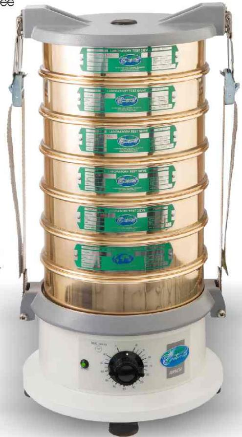
The low cost M100 is an excellent little laboratory shaker designed for 100 mm and 3" diameter sieves. It is robust, lightweight and provides the user with complete control over amplitude and vibration time.
